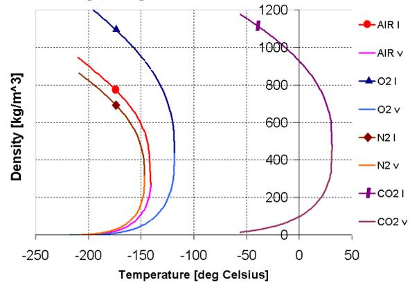
Fig. 1 Saturation densities of nitrogen, air, oxygen and carbon dioxide.
