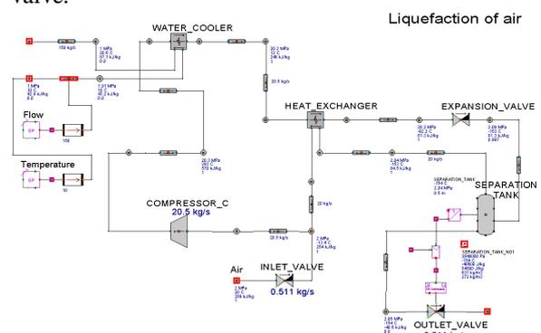
Fig. 2 Process model for the liquefaction of air.
