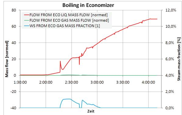
Fig. 7: Economizer parameters over start-up
