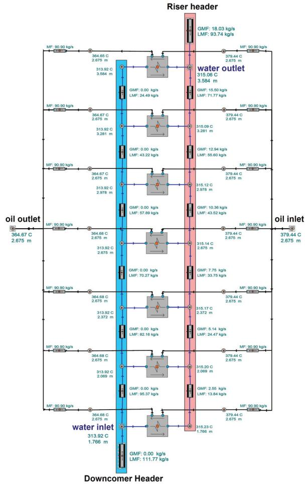
Fig. 3: layer discretization of steam generator 1
