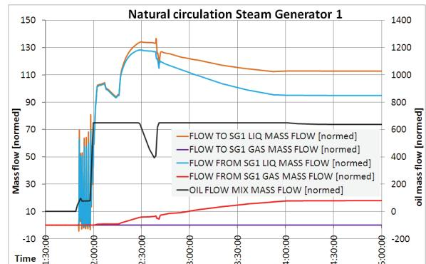
Fig. 8: Natural water circulation in Steam generator 1
