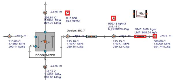
Fig. 2 View of the simulation interface GRADES
