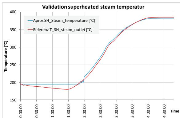
Fig. 5: Superheated steam temperature
