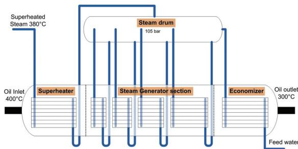
Fig. 1 Schema of the steam generation system
