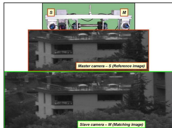
Fig. 7 Example of the stereo pair shots (target No. 13) – a part of the Catalogue of Targets
