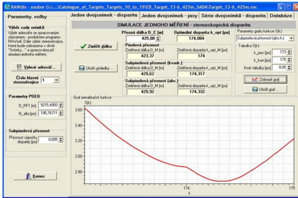
Fig. 11 Example of a course of the matching cost function  $S(k)$  for sub-pixel accuracy (SAD/MAD algorithm)
