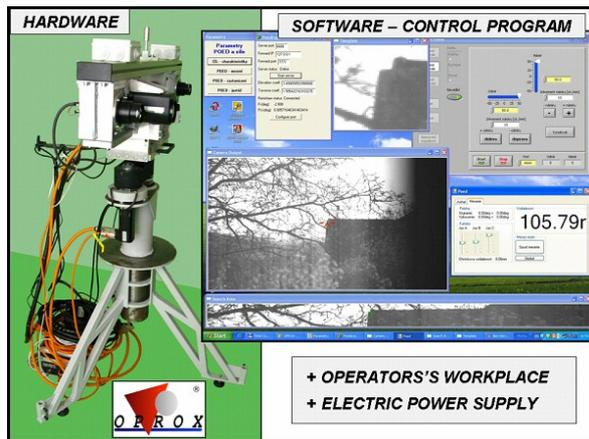
Fig. 1 Passive optoelectronic rangefinder (POERF) – the demonstration model 2009 [4, 5]
