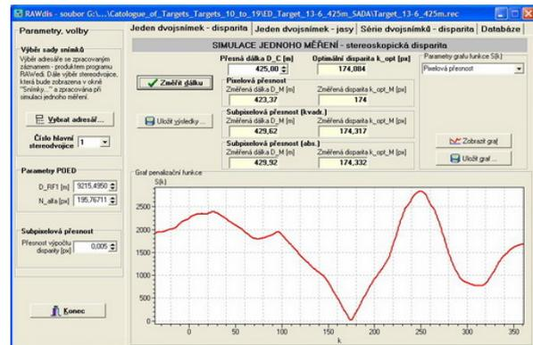
Fig. 9 The main window of the program RAWdis – the state after opening a file with shots from the Catalogue of Targets (the target No. 13) and after calculation of the target slant range estimate from one stereo pair images
