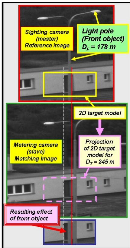
Fig. 17 The example of a front object influence on the creation of disconnected set of “effective” pixels on the 2D target model displaying the surface of the target No. 4 – a building
