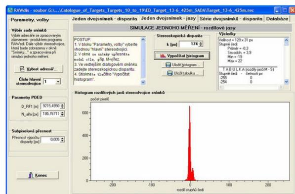
Fig. 10 The histogram of brightness differences on corresponding pixels after finding integer disparity of the target model (calculations for the area of the selected target model)
