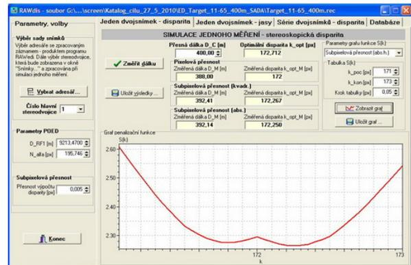
Fig. 21 Example of the course of the matching cost function  $S$  for finding sub pixel minimum
