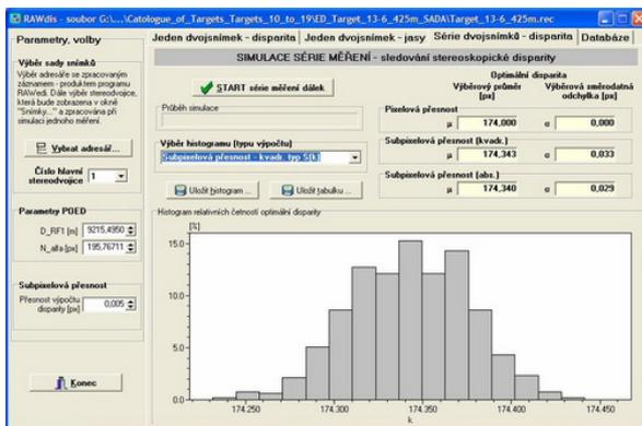
Fig. 12 The histogram of target slant range estimates (512 measurements) for the matching cost function generated from squared intensity brightness differences (SSD/MSE) on areas of the target model and the matching image (Fig. 10)
