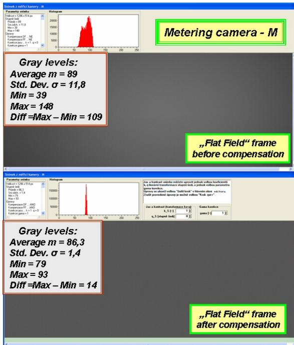
Fig. 20 Example of systematic errors compensation in the image record by the procedure described in the section 3.2 (“Flat Field” frame was randomly chosen from the set of 512 pair shots taken in September 4, 2009 – sky flats)
