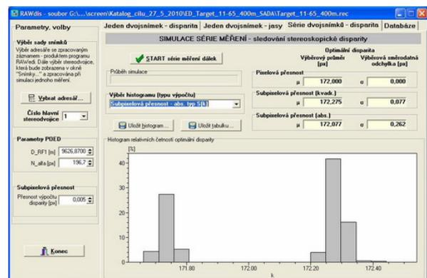
Fig. 22 Example of the effect of the spatial noise on the histogram of “sub pixel” disparities determined by the SAD algorithm for the target No. 11 ( $D_T = 400$ m)
