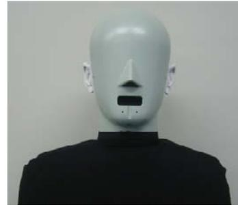
Fig. 6 Head and torso simulator with built-in microphones.
