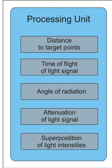
Fig.4: Architecture of the modular light propagation simulator
