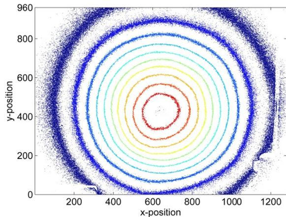
Fig.17: Colored light intensity distribution on different intensity levels (cuts through the figure 16)
