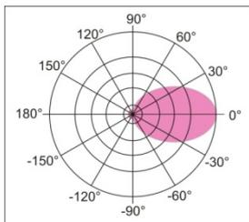
Fig.7: Example of a directional characteristic of a LED in polar coordinates
