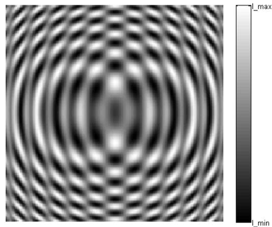
Fig.14: Simulated amplitude distribution of two AM-modulated microwave emitting exciters (coherent light sources)
