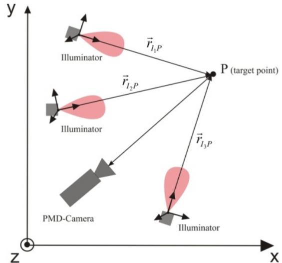
Fig.2: Example of a scenario with three different illuminators and one PMD-camera (PMD-sensor)
