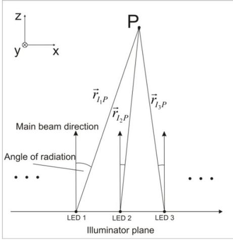
Fig.5: Illustration of an illuminator–target point configuration with respect to the light propagation
