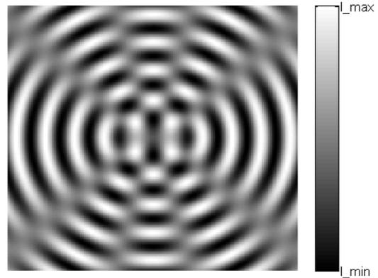
Fig.11: Simulated amplitude distribution of two microwave emitting exciters (coherent light sources)
