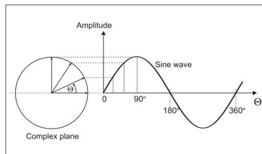
Fig.12: Conversion: sine-wave ↔ vector form
