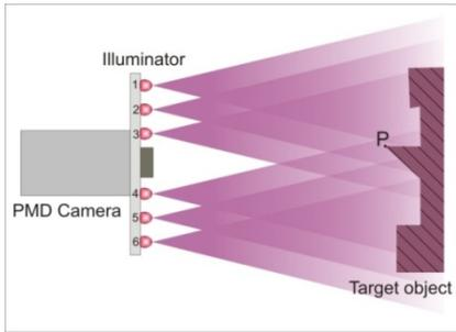
Fig.6: Moiré effect due to the non-uniform illumination
