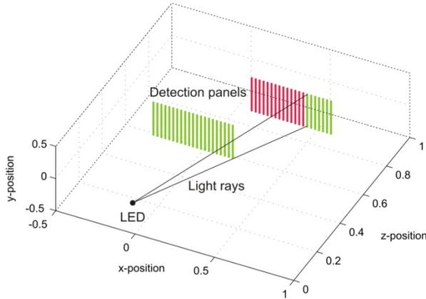
Fig.3: Arrangement of an illuminator and detection panels in a simulation environment
