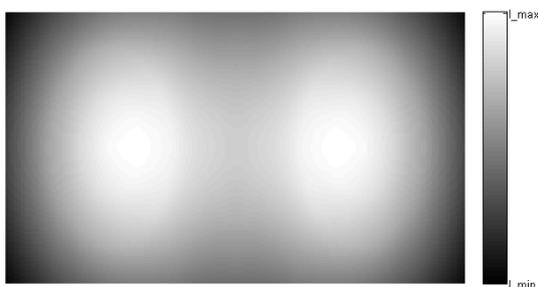
Fig.10: Simulated light intensity distribution of two incoherent light sources
