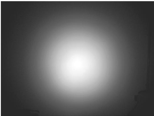
Fig.15: Measured distribution of the light intensity
