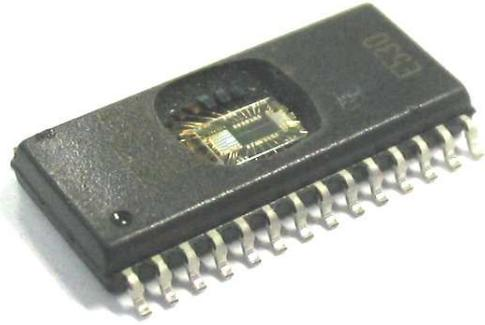
Fig. 4 View on the packaged test device (molding compound partially removed above the test chip) [8]
